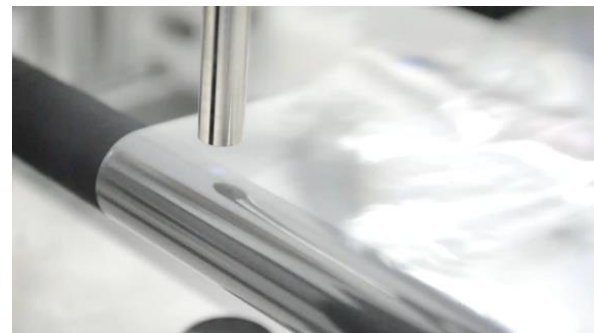
Figure 1: Real-time thickness measurement of PET film
