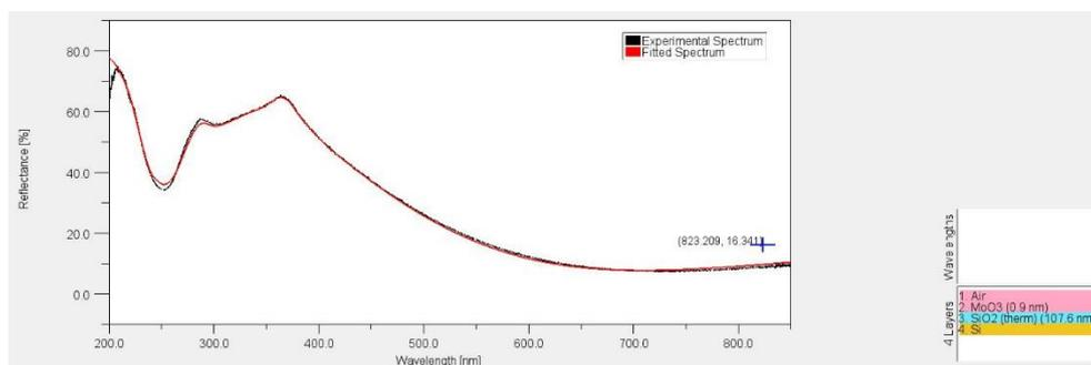
**Figure 2.** Experimental and fitted reflectance spectra of MoO<sub>3</sub> on top of a SiO<sub>2</sub> film, at the 200-850nm wavelength range.
