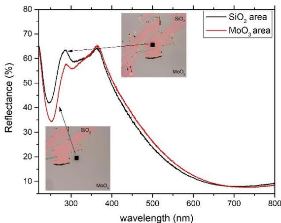
**Figure 1.** Absolute reflectance spectra of MoO<sub>3</sub> and SiO<sub>2</sub> film, obtained at the microscopic areas as shown in the inset images.
