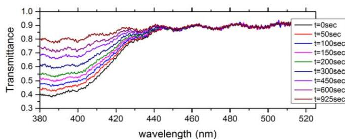
Figure 1: Transmission spectrum of the AZ5214 resist film after certain time exposures to room light
